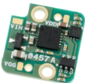
X-MW block Bias and Control
